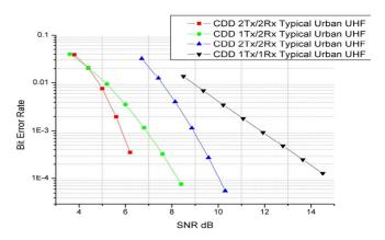
Figure 1 BER vs. SNR with Cyclic Delay Diversity
