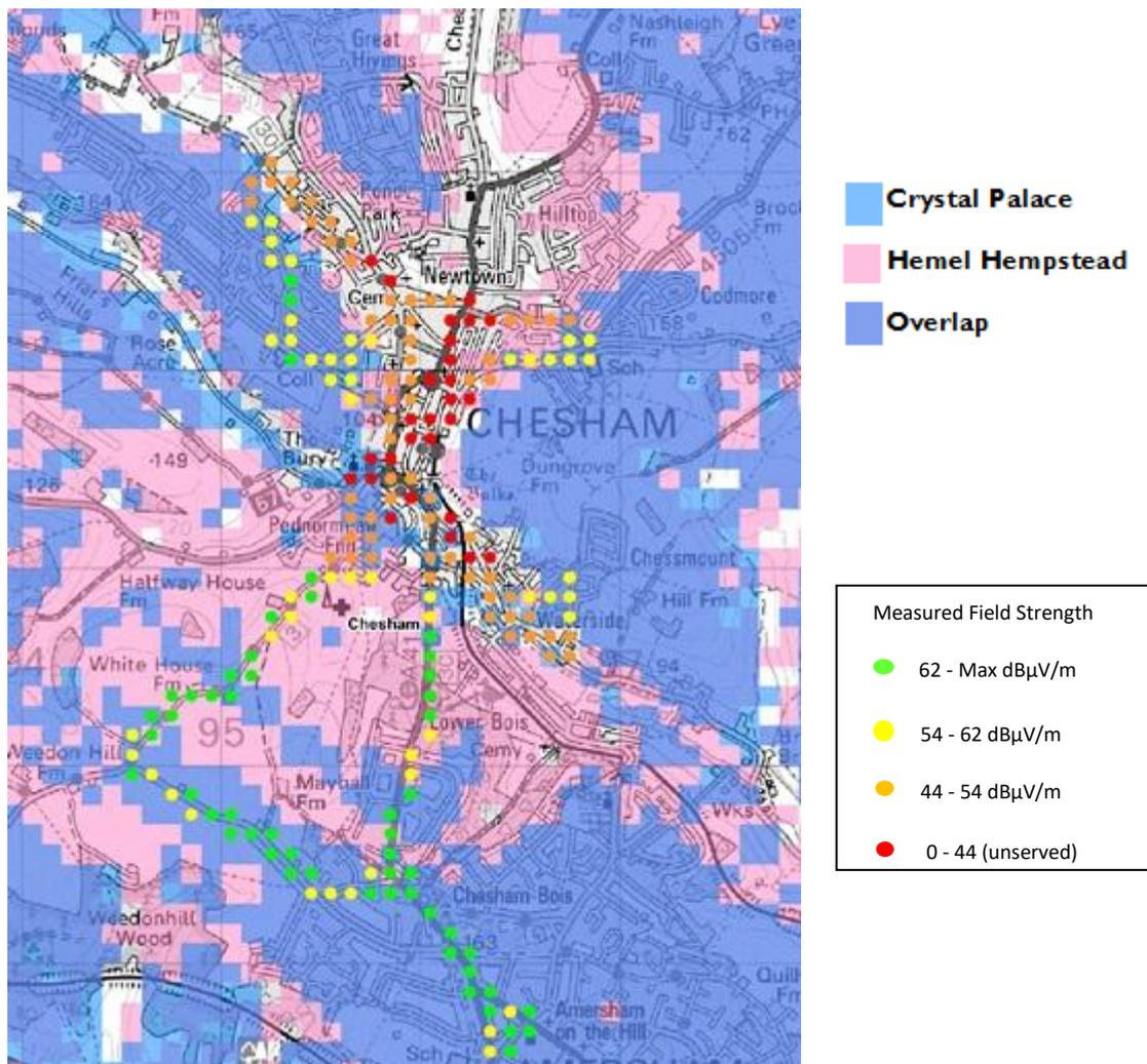
Figure I3: Predicted mobile coverage for channel 11D in Chesham from the two dominant servers, Crystal Palace and Hemel Hempstead (Gross transmitter coverage - No SFN gain). Drive survey measured Field Strength for channel 11D is also shown (measured at 1.5 m a.g.l. and averaged into 100 m pixels)
