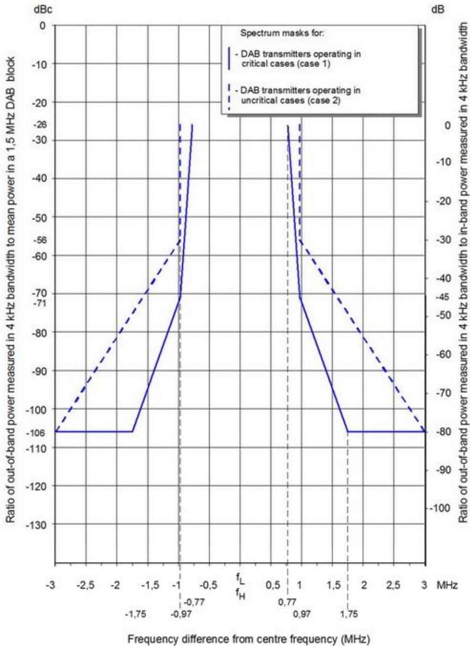
Figure 5: Spectrum masks for DAB out of band radiation
