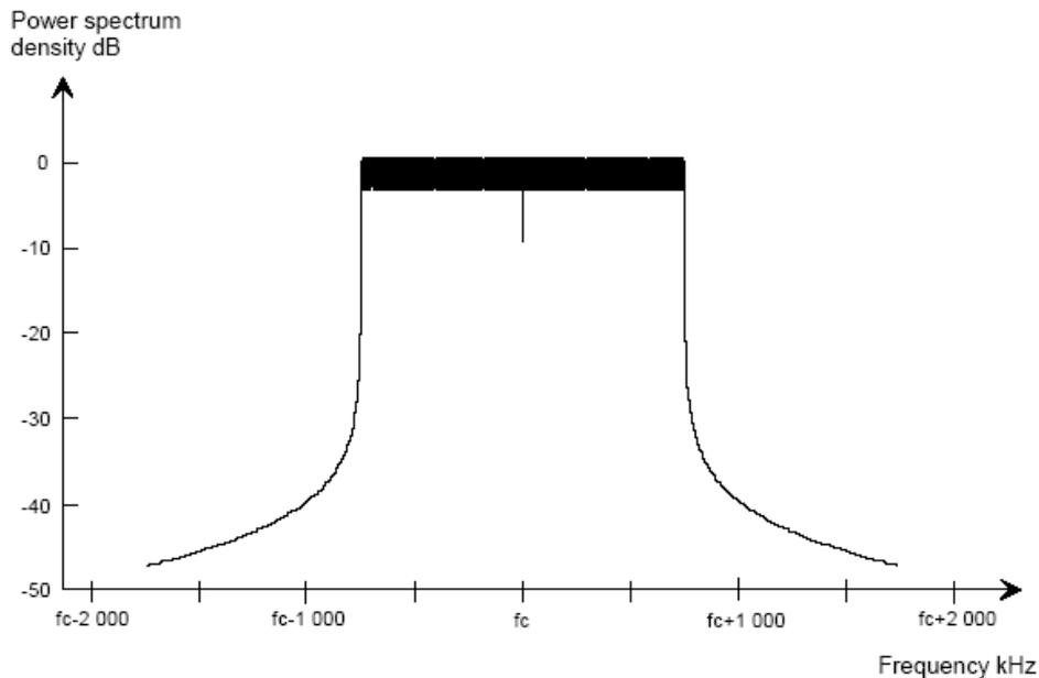
**Figure 2: DAB transmission signal spectrum (1.536 MHz channel)
