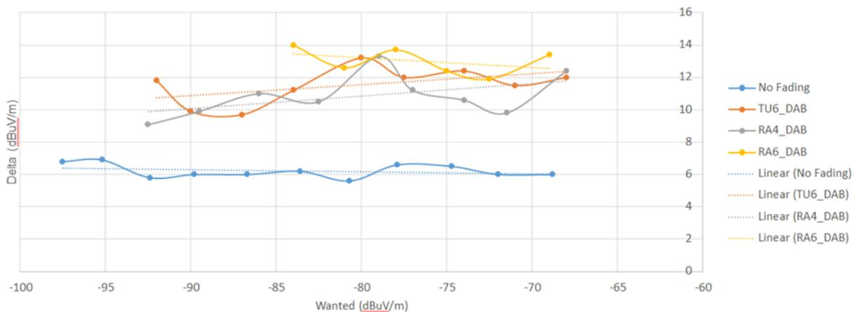
Figure 8: Protection ratio requirements for a range of channel types
