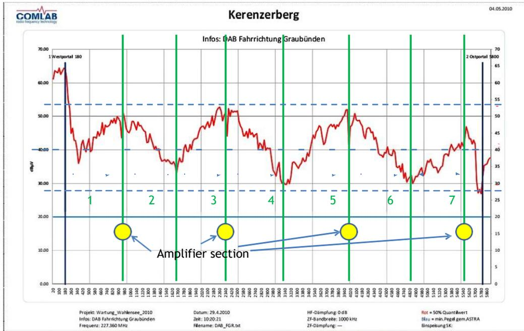
**Figure J2: Sample measurement for minimum coverage criteria for DAB**
