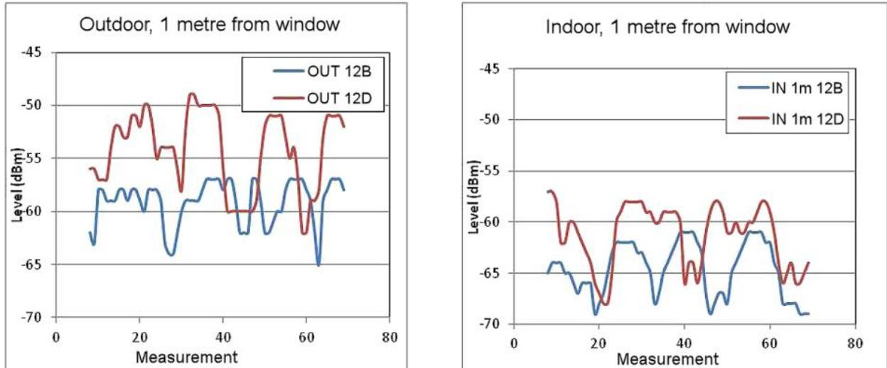
Figure E9: Indoor and outdoor signal measurements of channels 12B and 12D
