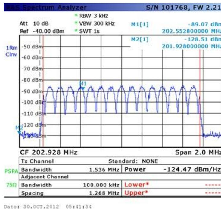
Figure 7: the spectrum of two equal power DAB signals combined with 10  $\mu$ s delay
