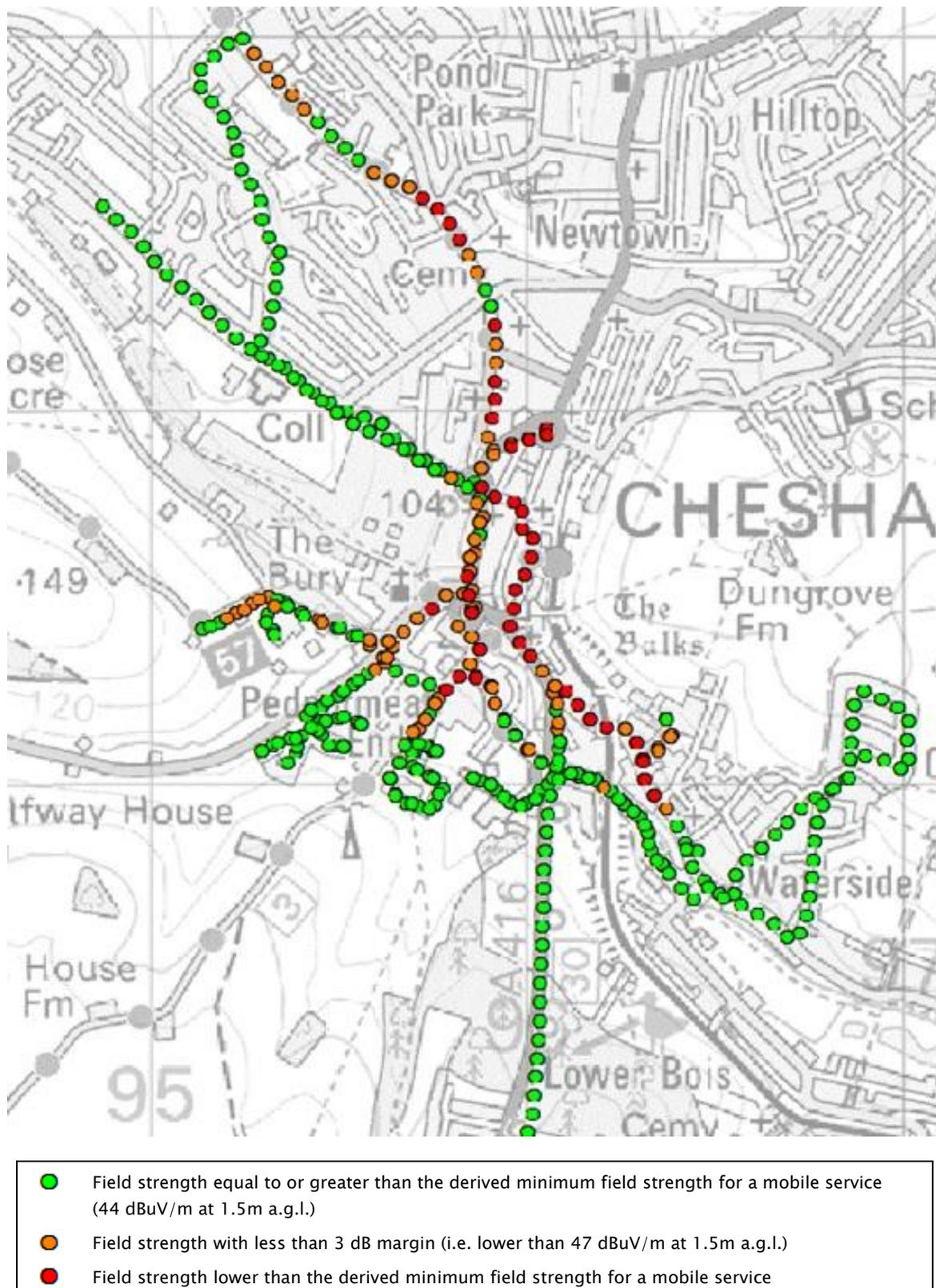
**Figure I8: Measured field strength data for the channel 11D service in Chesham before any ACI but showing areas considered unserved for a mobile service.**
