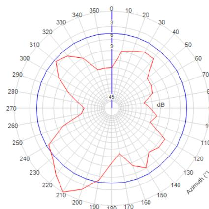
Figure C3: Typical in-glass antenna patterns
