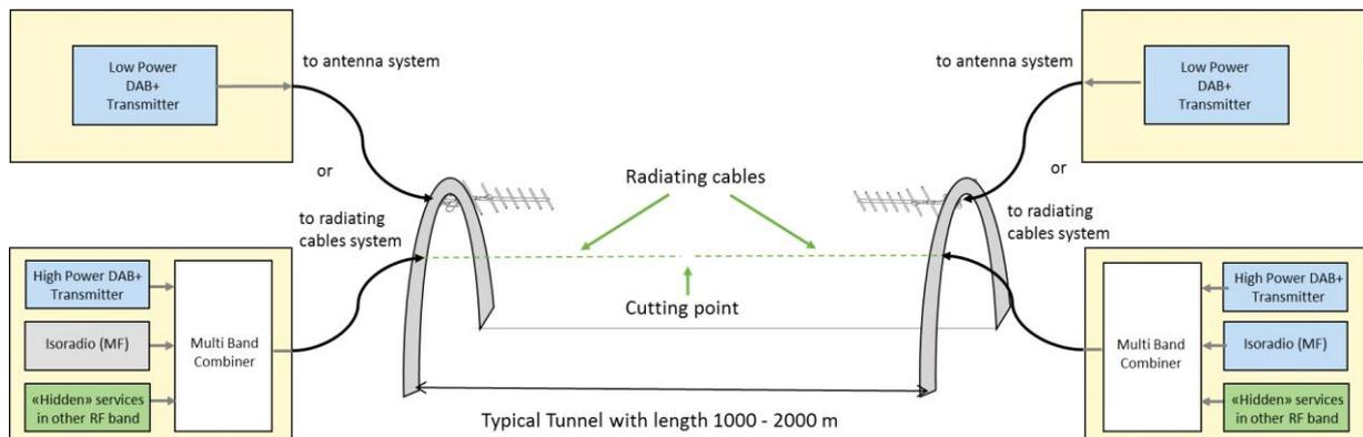
Figure J3: Radiating cable VS directive antenna
