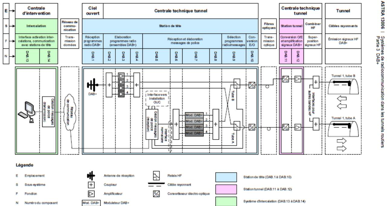
Figure J1: Overview of a DAB tunnel-system (courtesy of Swiss Federal Roads Authority)
