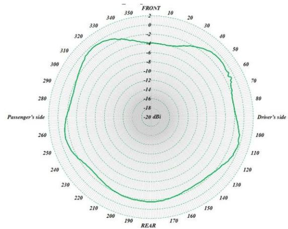
Figure C1: 'Ideal' Quarter wave monopole on car roof
