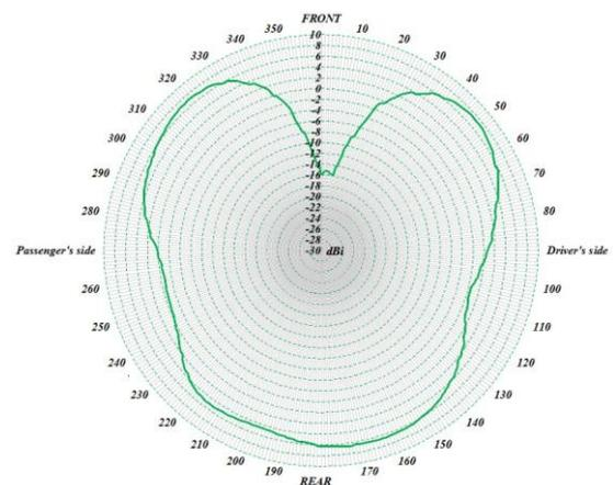
Figure C2: Quarter wave slant whip on car roof
