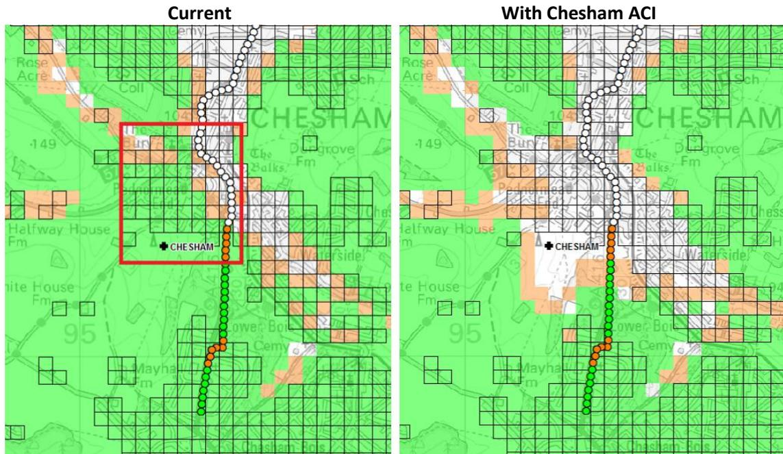
Figure 19: Predicted indoor coverage overlaid with surveyed field strength corresponding to ■ good and ■ robust indoor reception, and with  populated pixels
