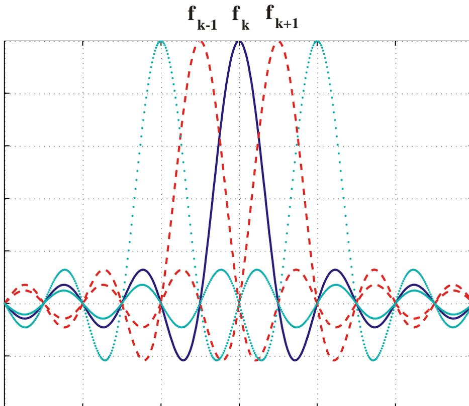
Figure 1: Schematic presentation of carrier orthogonality in an OFDM signal (after windowing)
