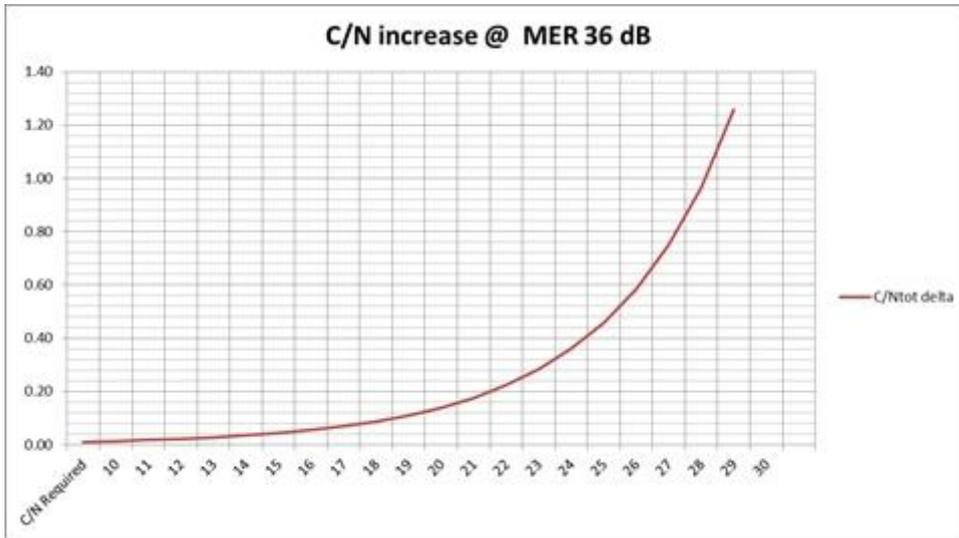
Figure 11: C/N degradation as a function the of required C/N value assuming a transmitter MER of 36 dB
