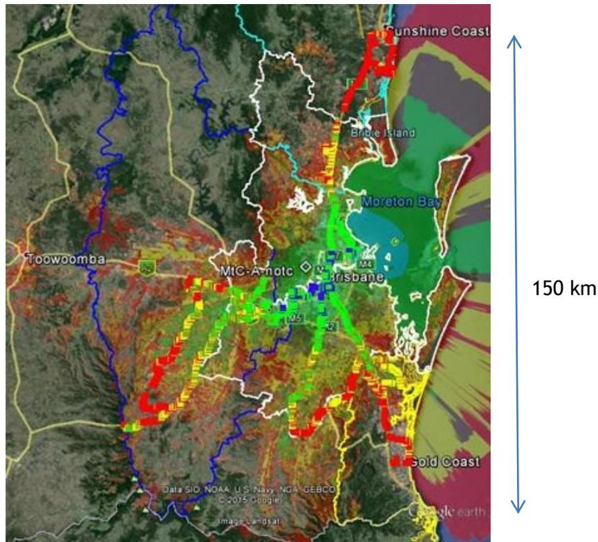
Figure F2: Coverage prediction after tuning with measurement overlay
