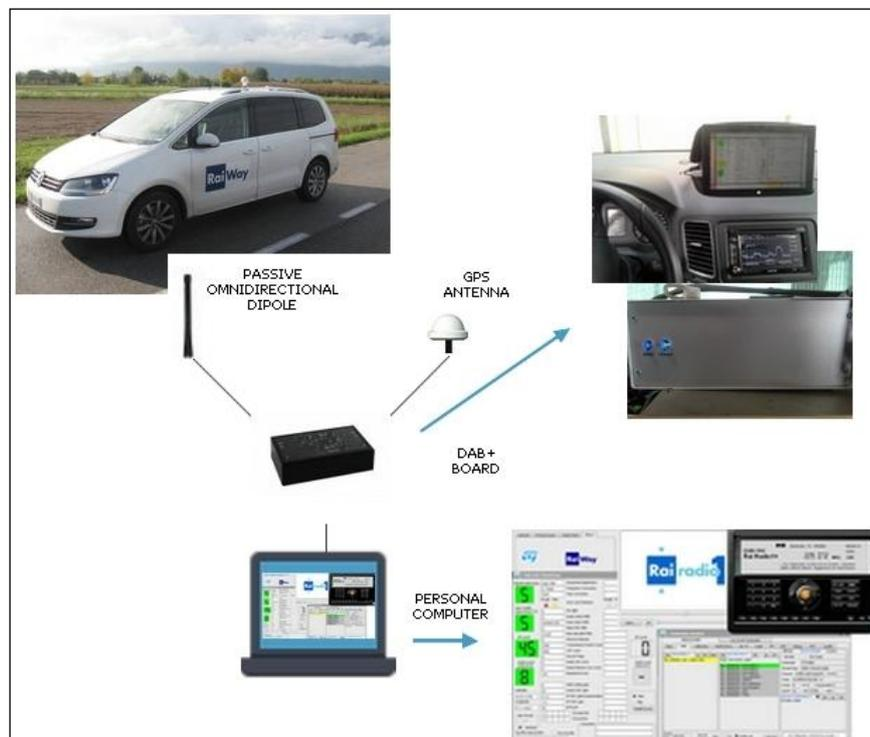
Figure H2: Measurement set up
