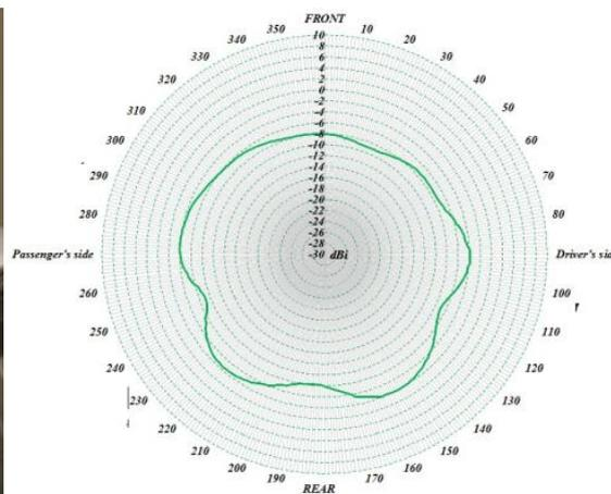
Figure C3: Shark's fin antenna on car roof
