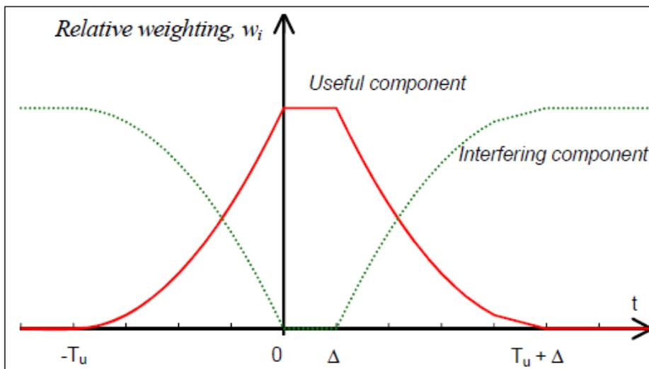
Figure 6: DAB model - splitting of a generic signal power into useful and interfering components
