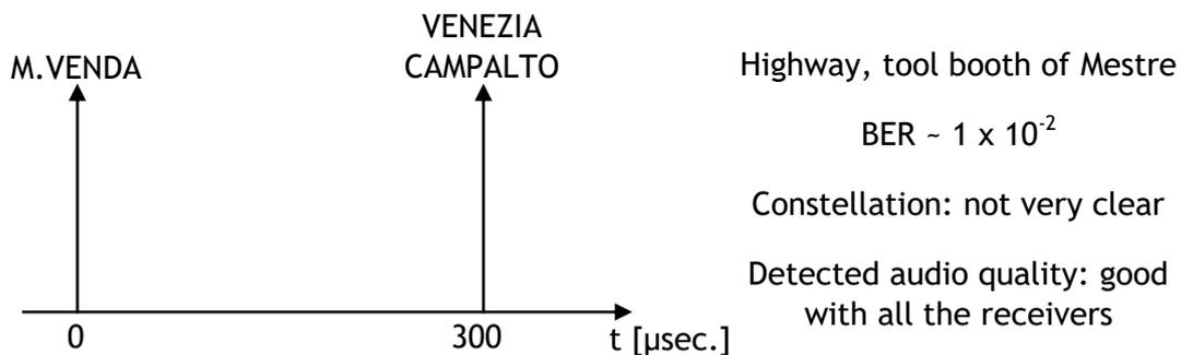
**Figure H4: Reception at Mestre from the two transmitters in test (300 μs delay)**
