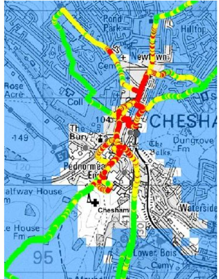
Figure I6: Predicted mobile coverage and channel 11D BER with 2nd Adjacent Channel Interferer at 100 W ERP
