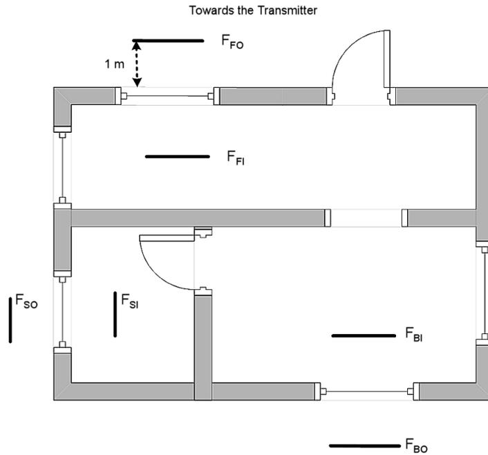
Figure E3: Field strength measurement points inside and outside a building
