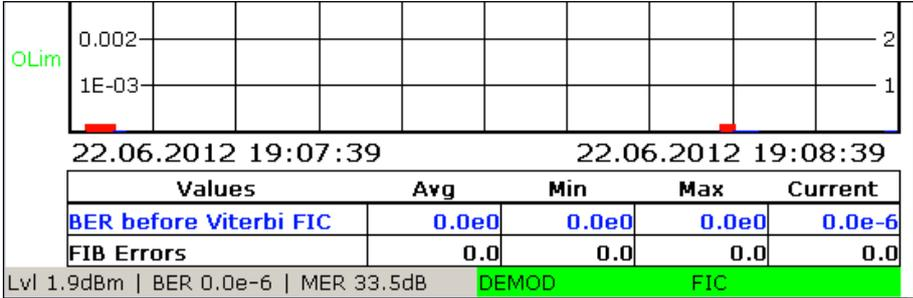
Fig. 15: TV/radio analyzer/receiver mode, MEAS→Measure Log menu: BER measurement with the measurement log. Red markers directly above the time axis (here in the 1st and 8th time segments) indicate a loss of synchronization. In this case, the BER measurement is invalid
