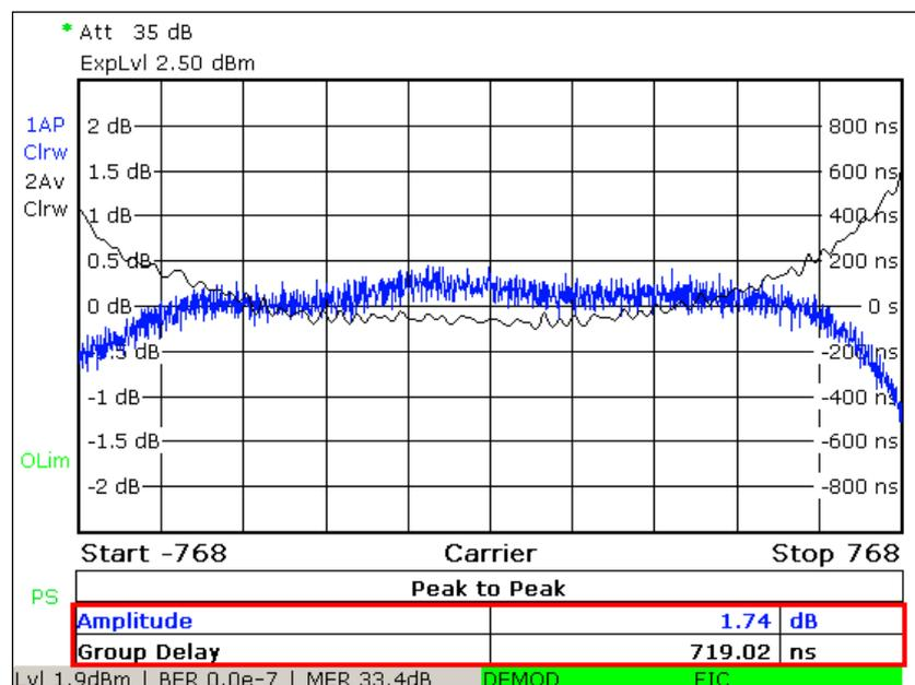
**Fig. 6:** TV/radio analyzer/receiver mode, MEAS→Channel Analysis→Amplitude & Group Delay menu: Amplitude frequency response and group delay after an uncompensated mask filter
