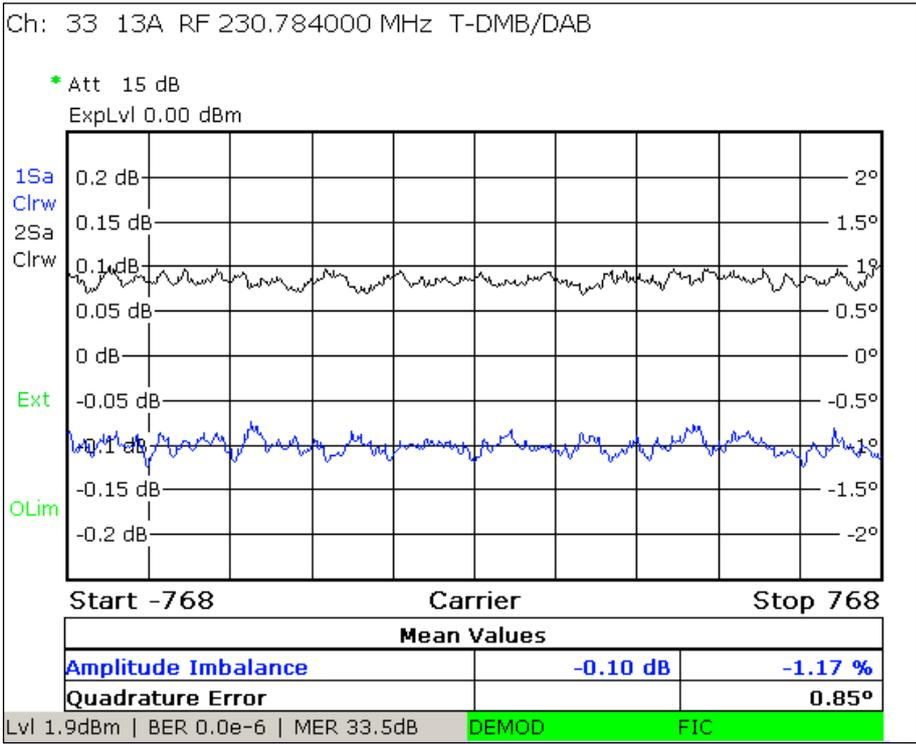
Fig. 5: TV/radio analyzer/receiver mode, MEAS→Modulation Analysis →I/Q Imbalance menu: Detailed analysis of amplitude imbalance and quadrature error over all carriers
