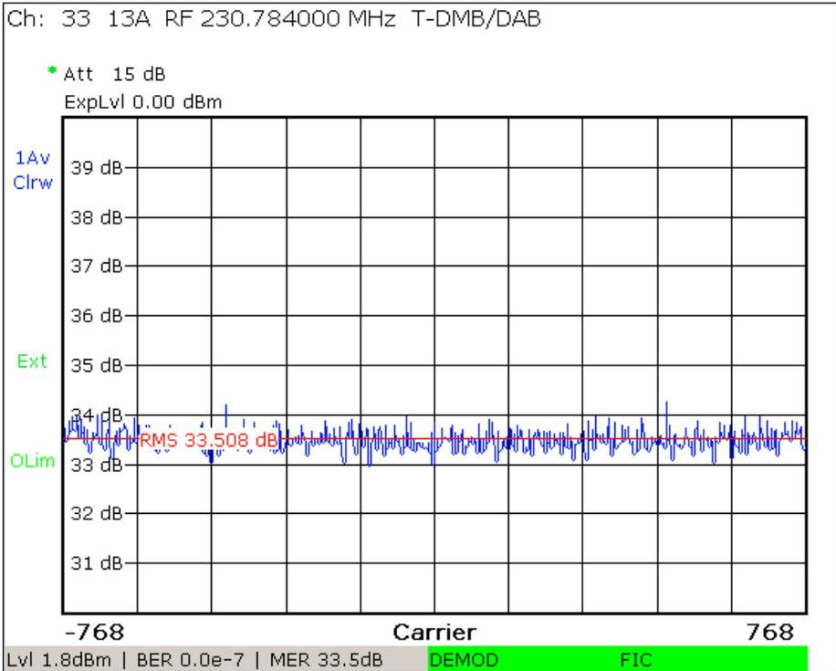
**Fig. 11:** TV/radio analyzer/receiver mode, MEAS→Modulation Analysis→MER(f) menu: MER as a function of the frequency and integration of the MER averaged over the channel (RMS).
