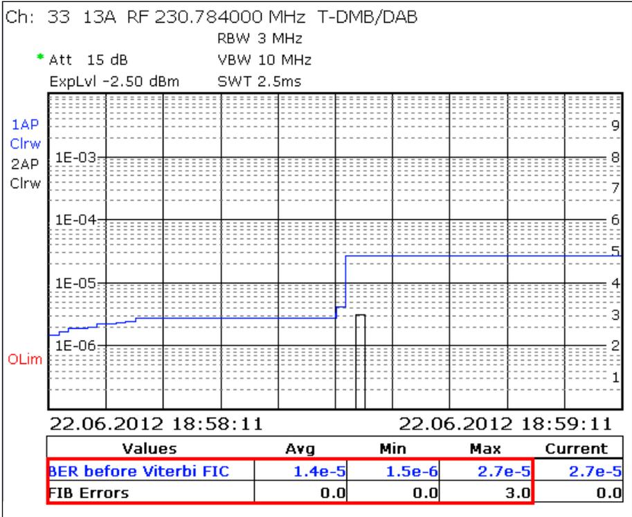
Fig. 16: TV/radio analyzer/receiver mode, MEAS→Measure Log menu: Valid BER measurement
