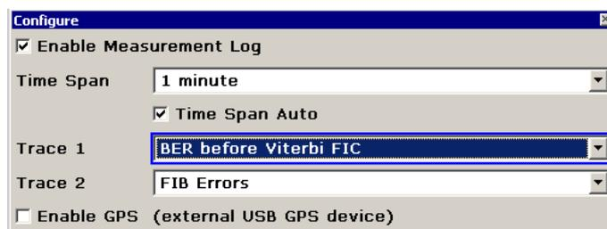
**Fig. 14:** TV/radio analyzer/receiver mode, MEAS→Measure Log→Configure menu: Configuration for the BER measurement
