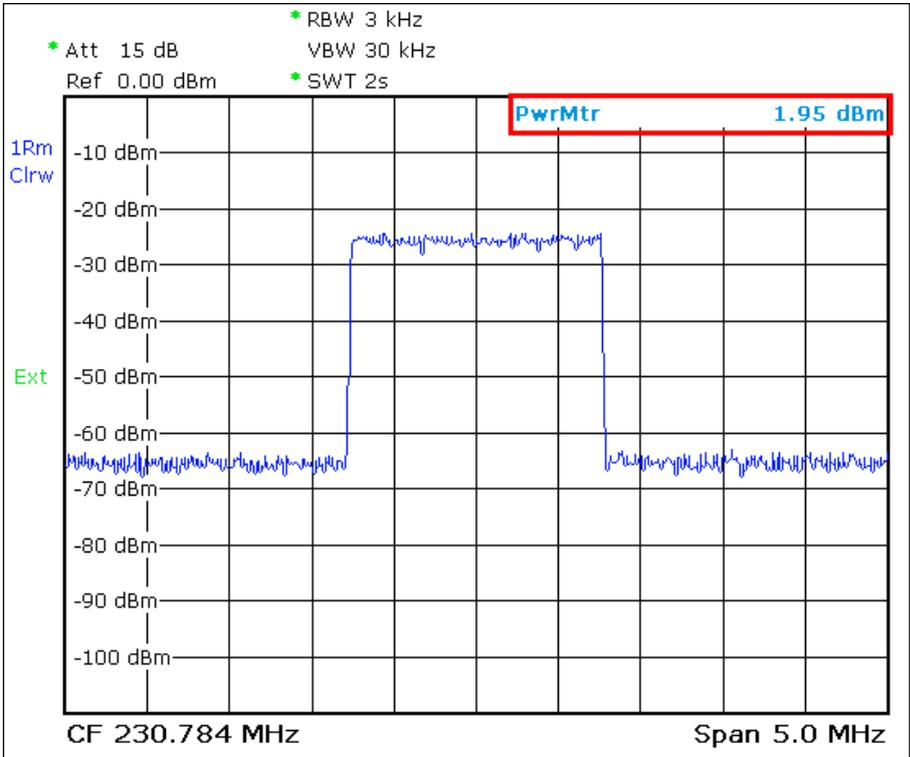
Fig. 3: Spectrum analyzer mode: DAB spectrum with integrated reading from the power sensor displayed at the top right
