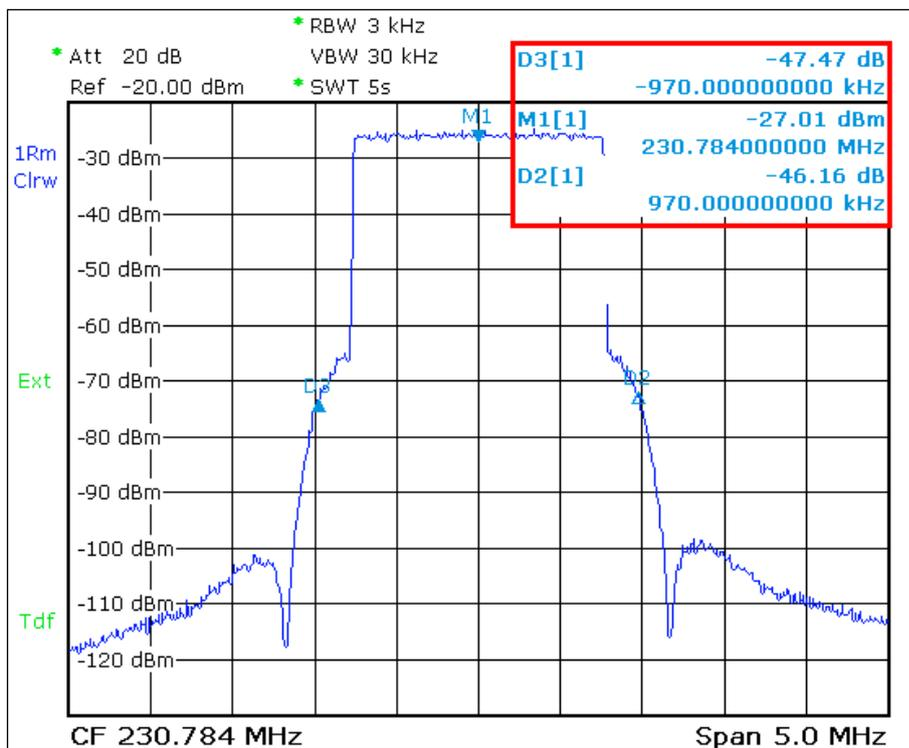
Fig. 7: Spectrum analyzer mode: Measuring the shoulder attenuation using the cursor method with active transducer file at +970 kHz in the 1.536 MHz DAB channel
