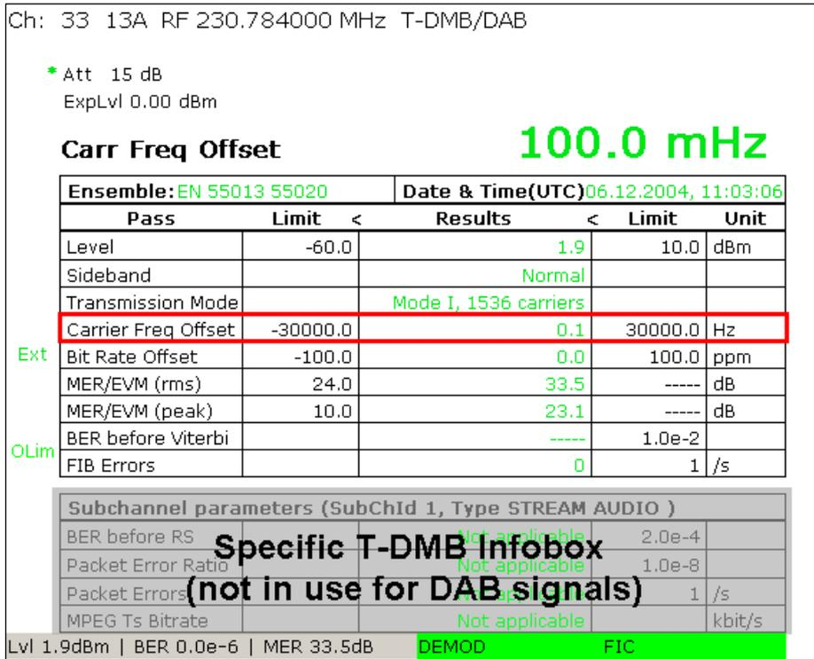
Fig. 10: TV/radio analyzer/receiver mode, MEAS→Overview menu: The frequency accuracy can be read in the 4th table row, as well as in the zoomed view (MEAS→Overview→Zoom)
